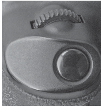
FIGURE 5.9 On Canon digital SLRs, the control wheel located just behind the shutter button allows you to automatically cycle through all reciprocal exposures after the camera has metered.
